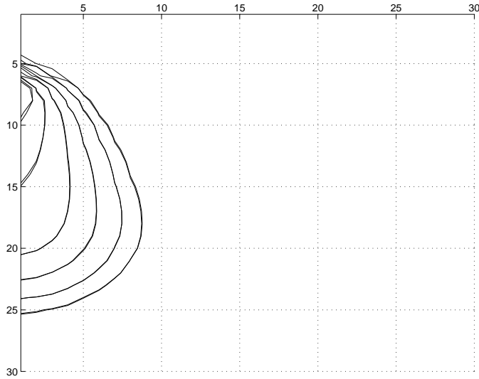
Figure 1.13. Concentration contours in the horizontal plane containing the solute source (layer 1) for three-dimensional solute transport in a uniform steady flow problem with CELDIS = 1 (14 time steps), NSC = NSR = NSL = 4 , NT = 4 .
